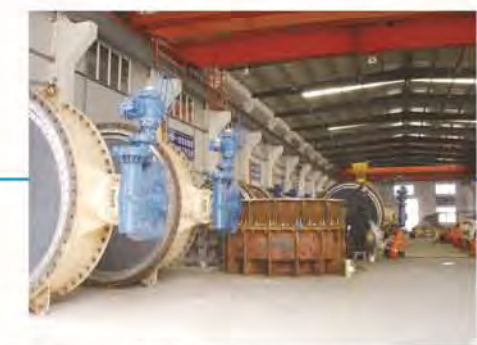
Butterfly Valve Assembling workshop
